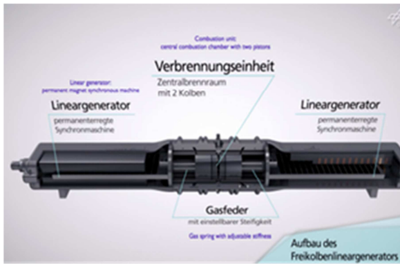
Figure 1. The DLR linear generator structure.
